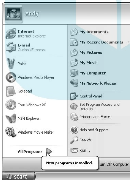
Figure 2-8: Most newly installed programs add themselves to the Start menu's All Programs area and announce their presence.
